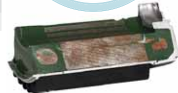
Insulated motor winding cross section
